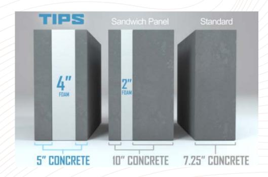
A material evaluation of the 4 inches of expanded polystyrene insulation and both wythes of concrete used in TIPS construction provides an R-value that exceeds the current energy code and the R-value of sandwich tilt-up walls that typically utilize 2 inches of insulation.
